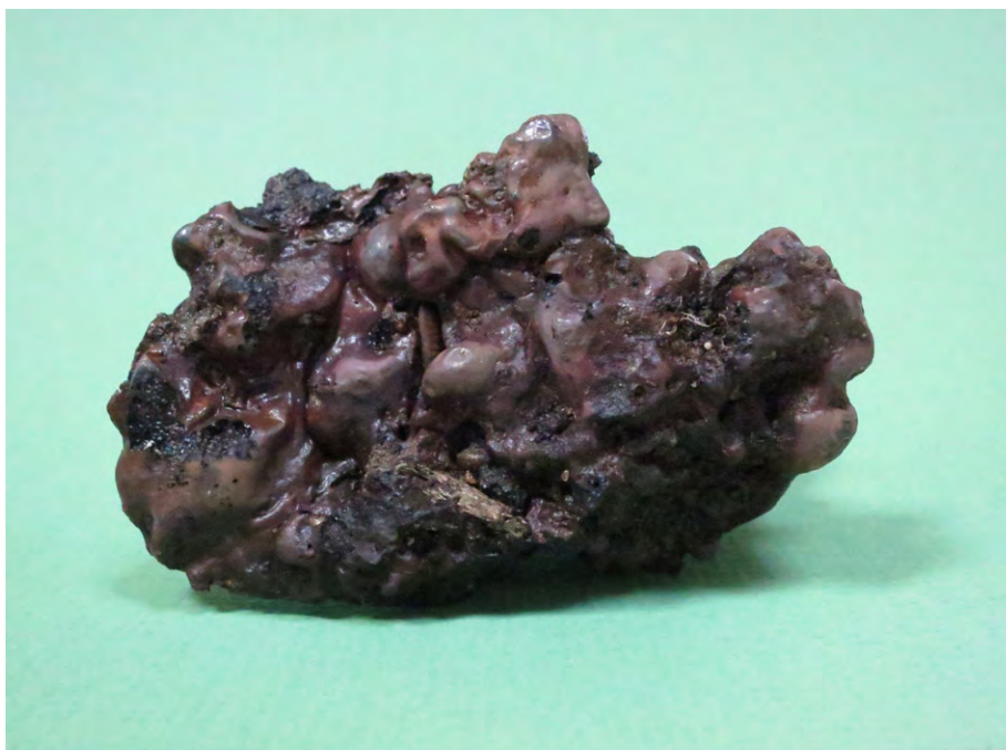
A clinker from a steam engine contains material that melted but didn't burn in the engine's coal bed. Since these blocked the
