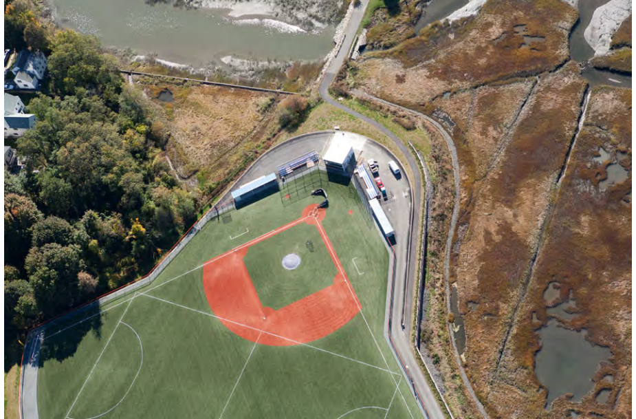
The Salem State Vikings baseball diamond from the air. Pickman Park can be seen in the background. The infield and outfield are both made from synthetic turf and cap a landfill. You will see four foot high standpipes around the property where the landfill is monitored. Courtesy of Rick Ashley.
